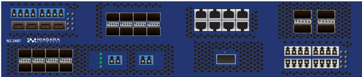
N2 2847 Front panel configured with (top row) two 1/10Gb bypass links, eight packet broker 1/10Gb ports, eight packet broker 1000BaseT ports, four 40Gb packet broker ports, (bottom row) 100Gb+8x10Gb bypass port, one 100Gb packet broker port, four link 1/10Gb passive tap
