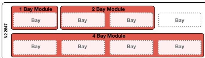
Each row in the 2847 chassis has four 1 width bays. User can dynamically hotswap different bay-width modules to mix and match module functionality and and module bay width size according to their needs. The double width bay module can dynamically fit into the space of any two adjacent 1 width bay locations as depicted above.
