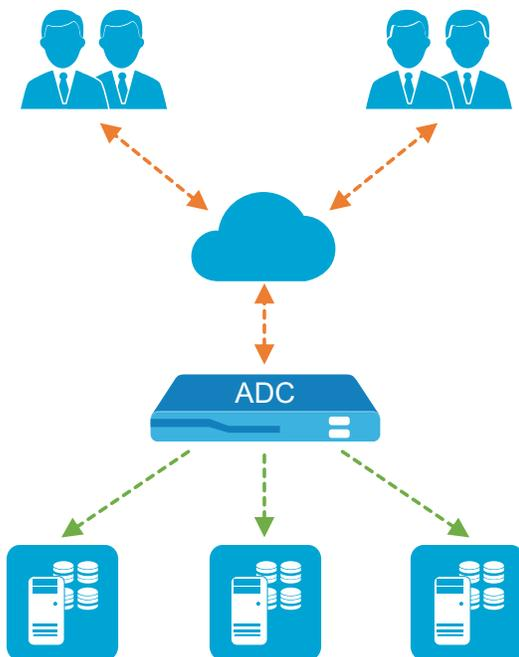
Figure 3: Server load balancing scenario
