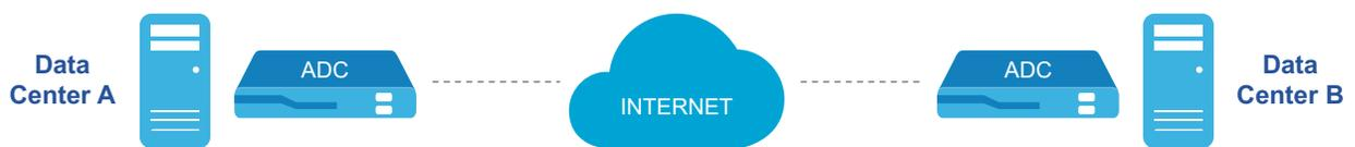
Figure 6: Hillstone's GSLB with SmartDNS intelligently routes traffic among multiple data centers.
