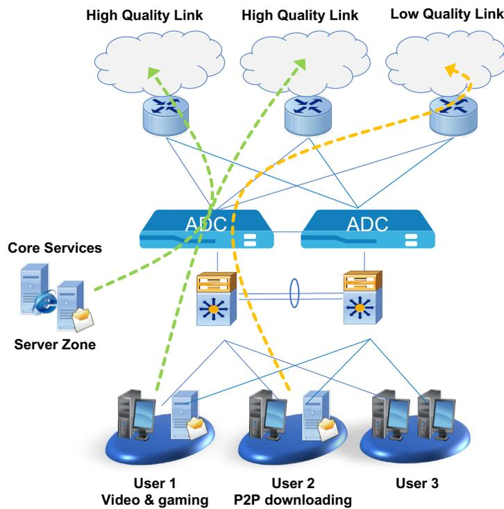
Figure 5: Link load balancing scenario – application-based routing
