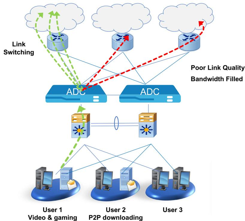
Figure 4: Link load balancing scenario – dynamic link switching
