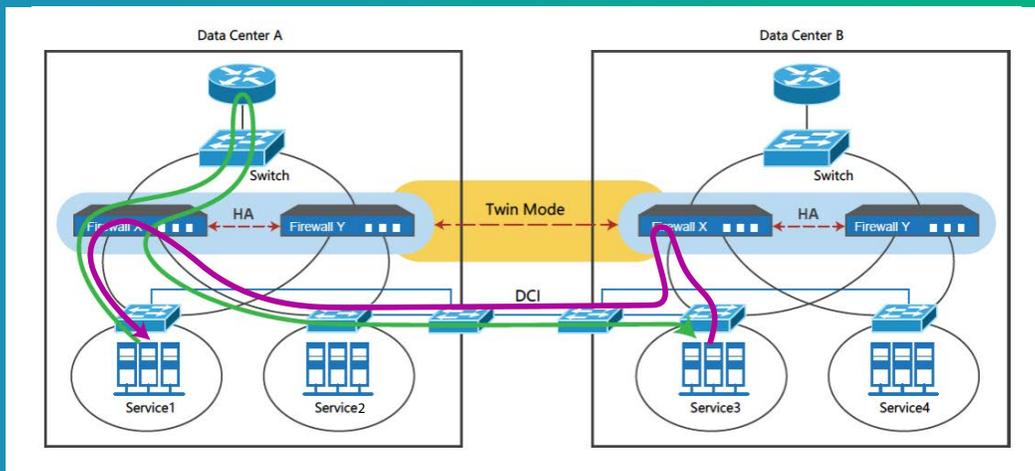
Figure 2: Illustrates how Firewall Twin-Mode would work in the same redundant data center scenario described above.
