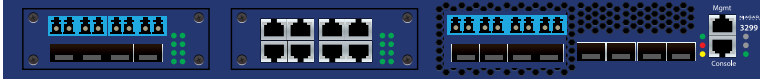
Figure 1: Rackmount populated with two modules with dual fiber bypass segments and one module with dual copper bypass segments. The right hand module with dual fiber bypass segment is fixed
